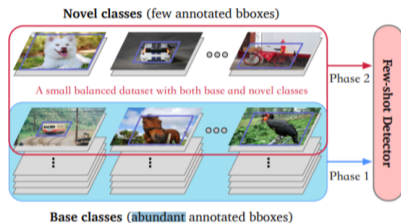
Figure 1: We propose a novel few-shot detection model that trains a basic detection model and a meta-model on base classes with sufficiently many samples in the first phase. In the second phase the meta-model is trained to fast adapt the detection model to detect novel objects by reweighing its intermediate features to be more discriminative and sensitive to the novel classes with a few examples.
